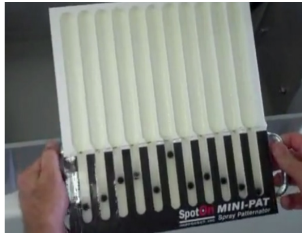
Patternator showing defective nozzle pattern. Source: Innoquestinc.com
