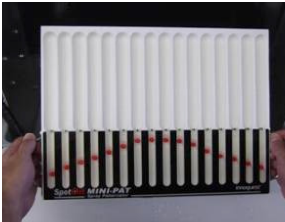
Patternator showing good nozzle pattern. Source: Innoquestinc.com
